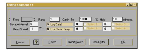
Ramp at 1 degree per minute to 1000 degrees; hold for 10 minutes; storage interval of 5 seconds; log data.
